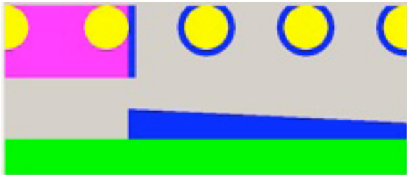
... this time with higher squeegee pressure and now an ugly thick edge to the print
