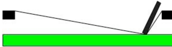
Edge of the mesh, relatively high pressure required, large distortion
