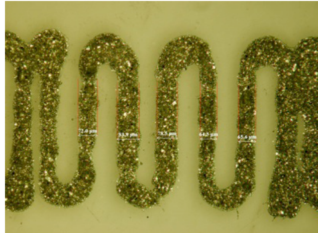
Our 50μm line becomes a 75μm line
