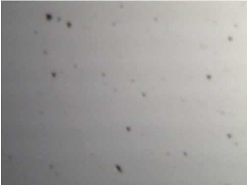
Splatter (dark spots on the white background) from a solid area (off to the left) that flew a long way
