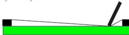
Lower snap-off (off contact) and relatively lower pressure/distortion
