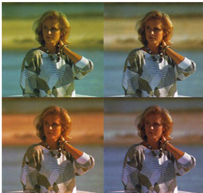
This portion of one of the Linotype-Hell test images shows the wide colour variation from four of the eight test sequences. Clockwise from the top left, 4:MCYK, 5:MYCK, 6:YCMK, 8:CMKY
