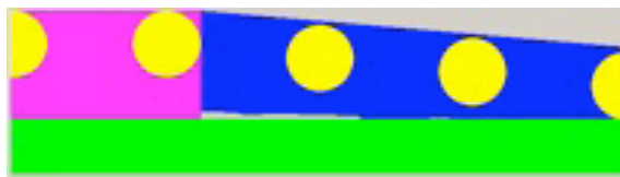
This thick stencil will give negative sawtoothing
