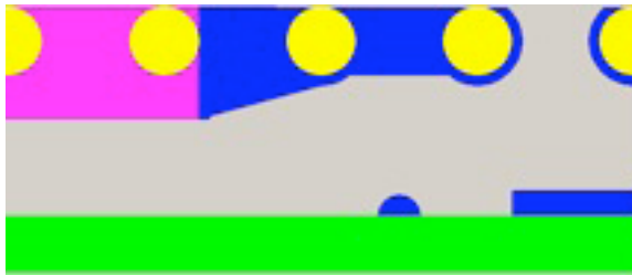
The ugly effect of a thick stencil and inadequate squeegee pressure
